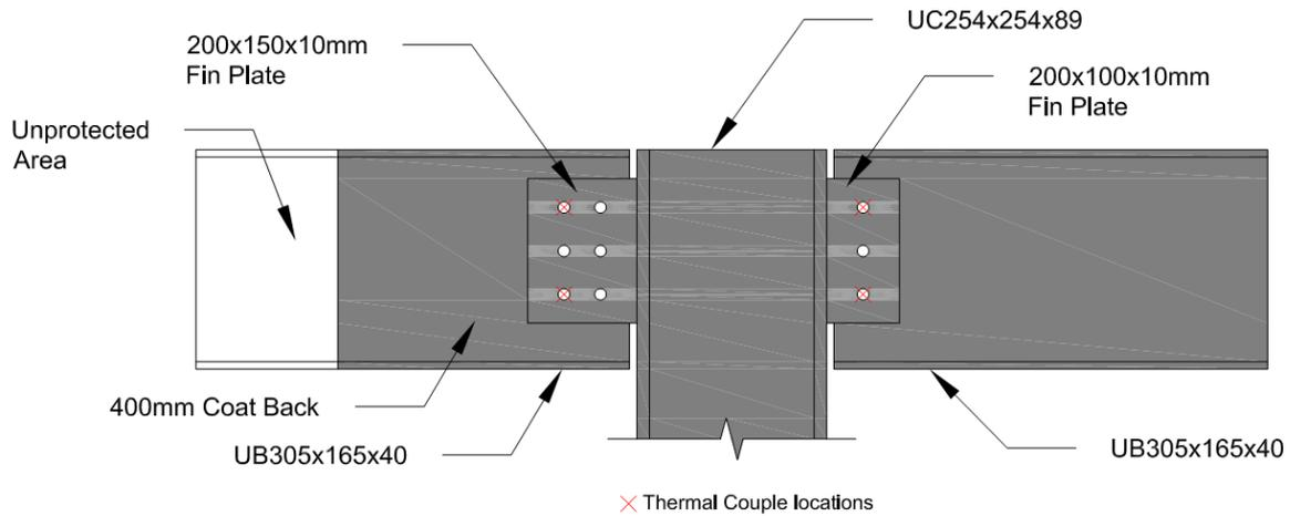
**(a) 400 mm coat back test configuration**
