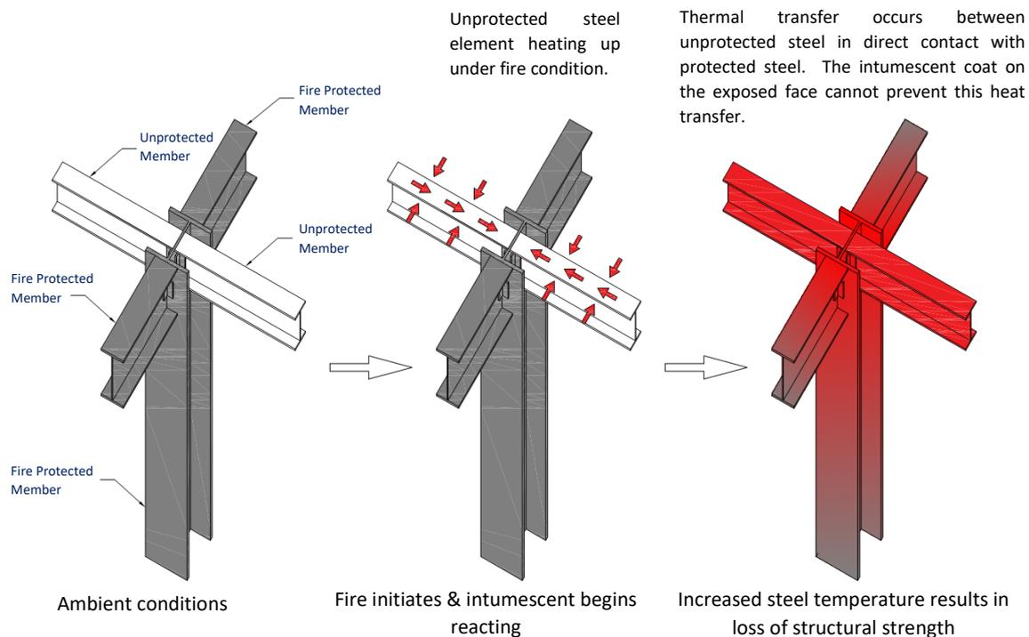
**Figure 1. Unprotected steel in contact with protected steel.**
