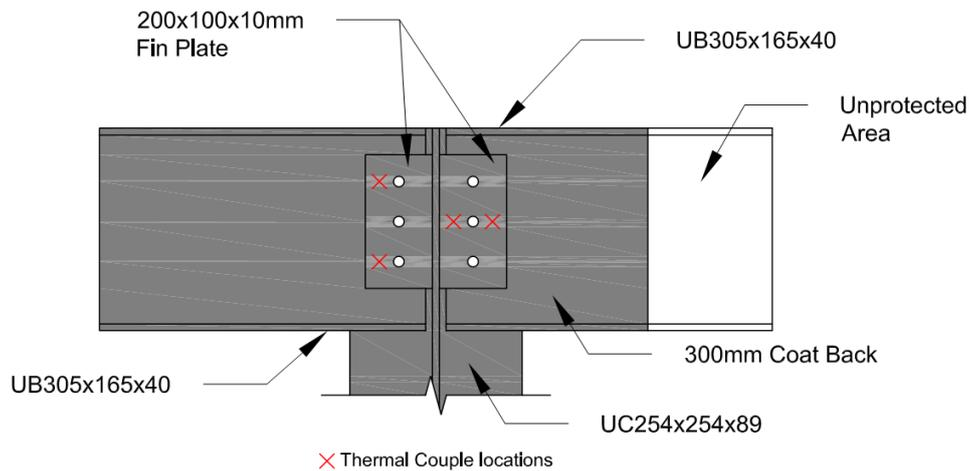
**(b) 300 mm coat back test configuration.**
